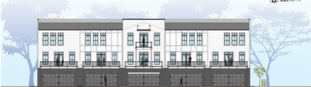
C TOWNHOME BACK ELEVATION - 2-CAR (5 UNITS) SCALE: 3/16" = 1'-0"
